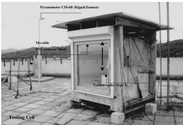
Fig. 10. Picture of testing cell.
